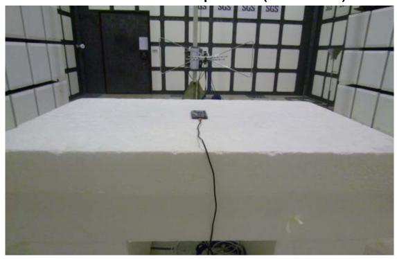
Radiated Emission Set up Photos (Above 1GHz)
