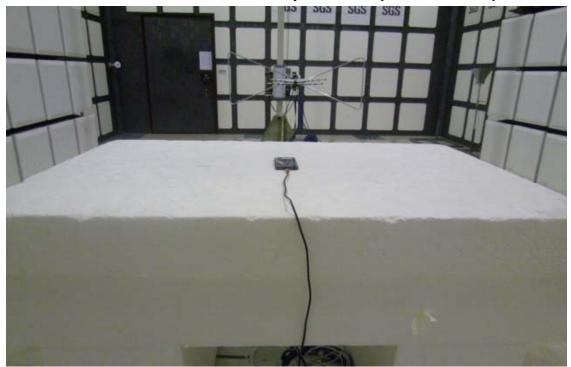
Radiated Emission Set up Photos (Above 1GHz)
