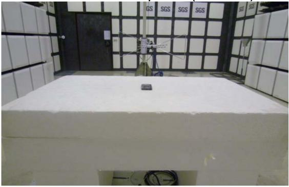
Radiated Emission Set up Photos (Above 1GHz)
