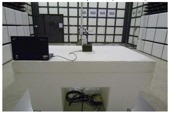
Radiated Emission Set up Photos (Above 1GHz)
