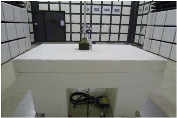
Radiated Emission Set up Photos (Above 1GHz)
