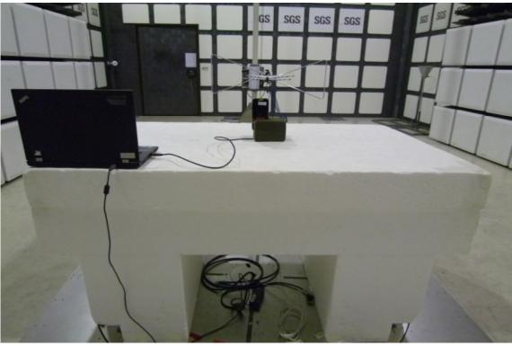
Radiated Emission Set up Photos (Above 1GHz)
