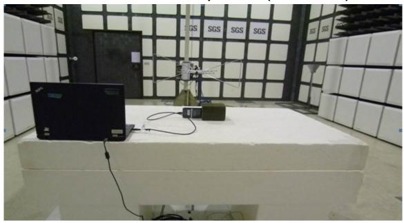
Radiated Emission Set up Photos (Above 1GHz)
