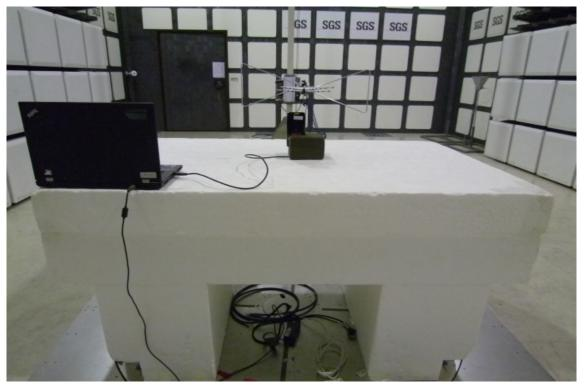
Radiated Emission Set up Photos (Above 1GHz)
