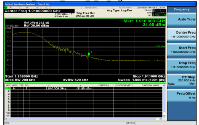
Band2 15MHz QPSK 1 74 HighCH19125-1902.5
