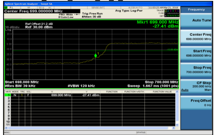
Band12 3MHz QPSK 15 0 HighCH23165-714.5
