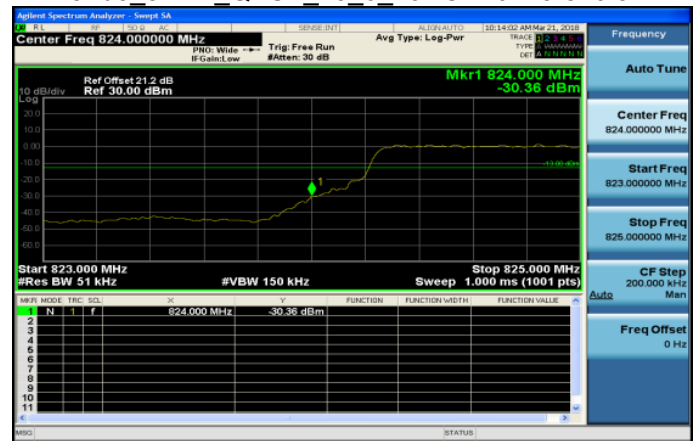
Band5 5MHz QPSK 25 0 HighCH20625-846.5
