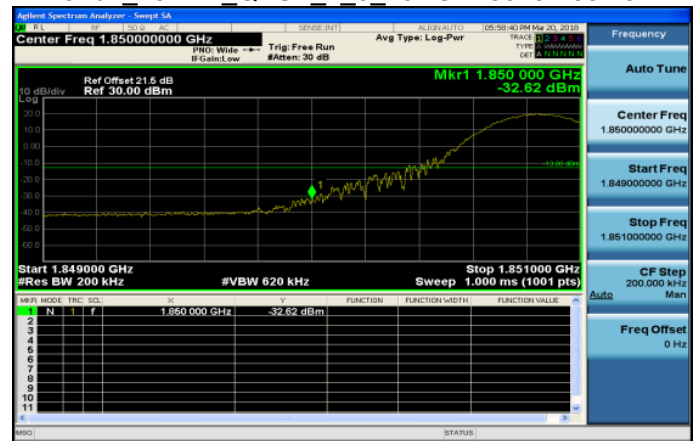
Band2 15MHz QPSK 1 74 HighCH19125-1902.5
