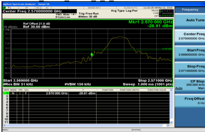
Band38 5MHz QPSK 1_24 HighCH38225-2617.5
