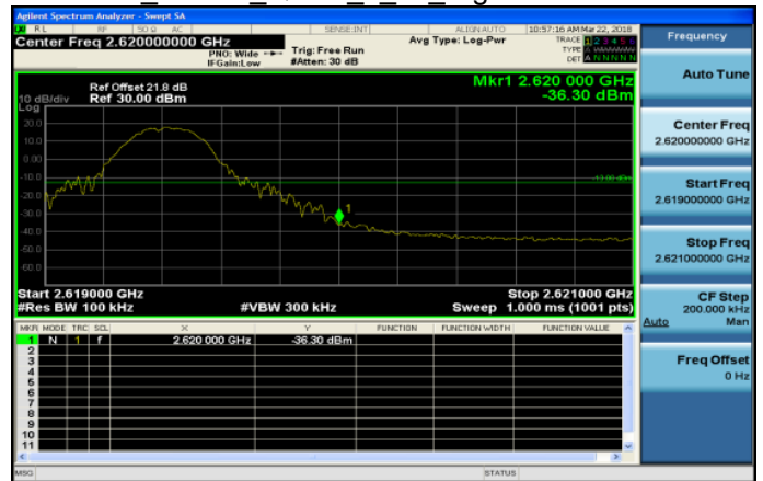
Band38 10MHz QPSK 1_49 HighCH38200-2615
