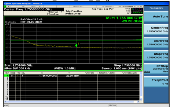
Band4 20MHz QPSK 100 0 HighCH20300-1745
