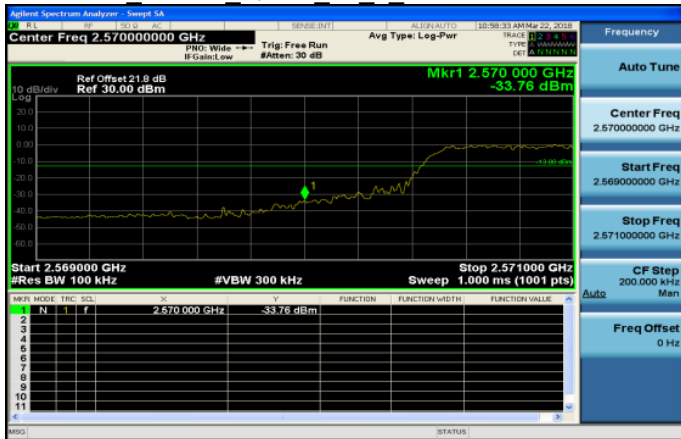
Band38 10MHz QPSK 50 0 HighCH38200-2615
