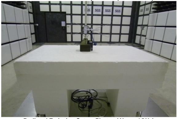
Radiated Emission Set up Photos (Above 1GHz)
