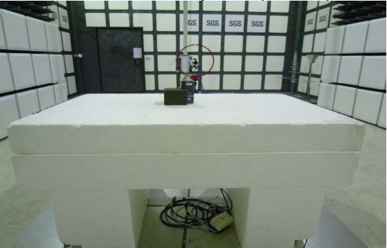
Radiated Emission Setup Photos (30MHz~1GHz)
