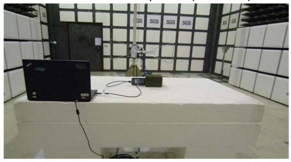
Radiated Emission Set up Photos (Above 1GHz)
