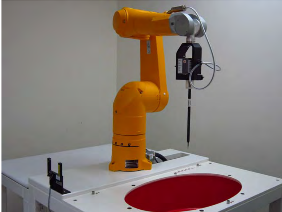
Fig.1 Photograph of the SAR measurement system
