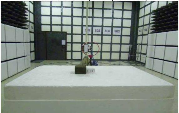
Radiated Emission Setup Photos (Below 1GHz)
