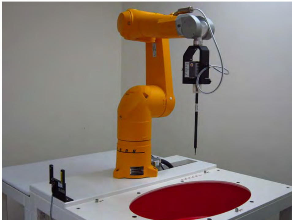
Fig.1 Photograph of the SAR measurement system
