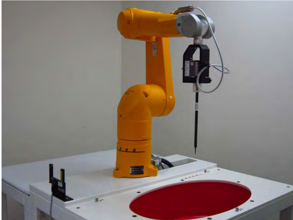
Fig.1 Photograph of the SAR measurement system
