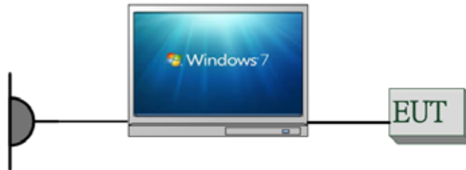
Fig. 2-2 Radiated Emission Configuration (NFC)
