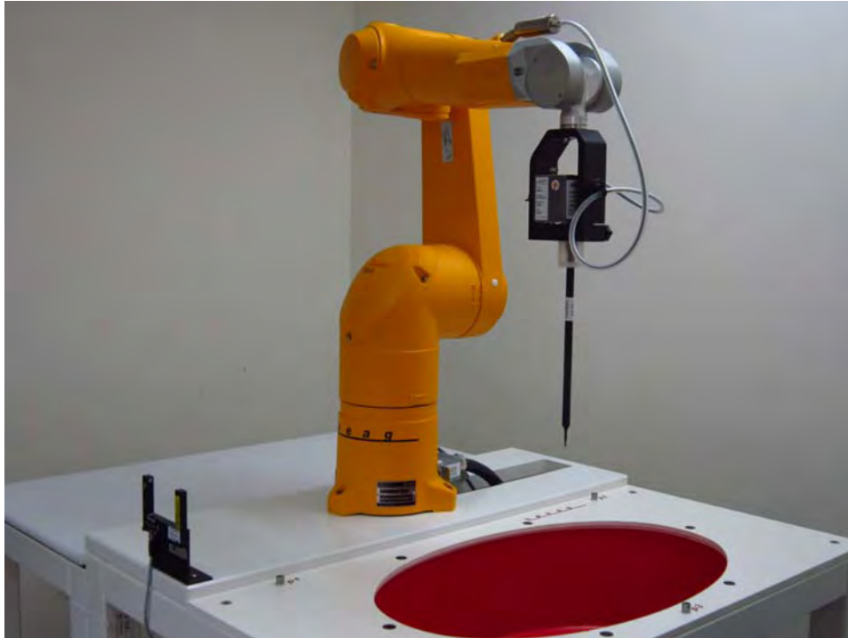
Fig.1 Photograph of the SAR measurement system
