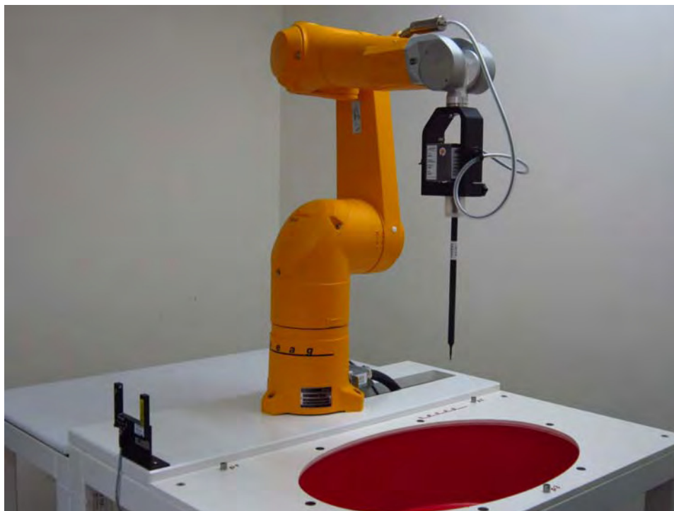
Fig.1 Photograph of the SAR measurement system
