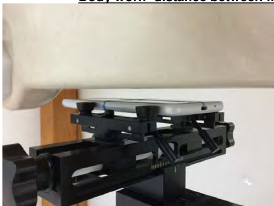
Fig.7 EUT Front side to flat phantom
