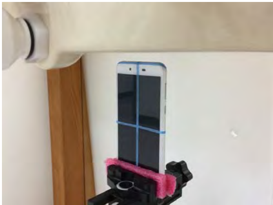
Fig.11 EUT Top side to flat phantom
