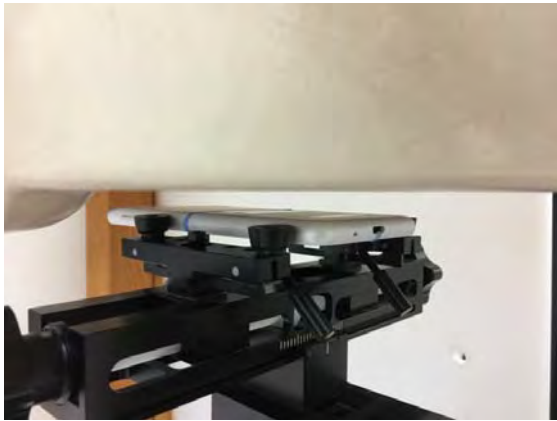
Fig.10 EUT Back side to flat phantom
