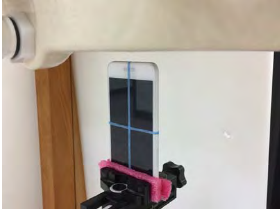
Fig.12 EUT Bottom side to flat phantom
