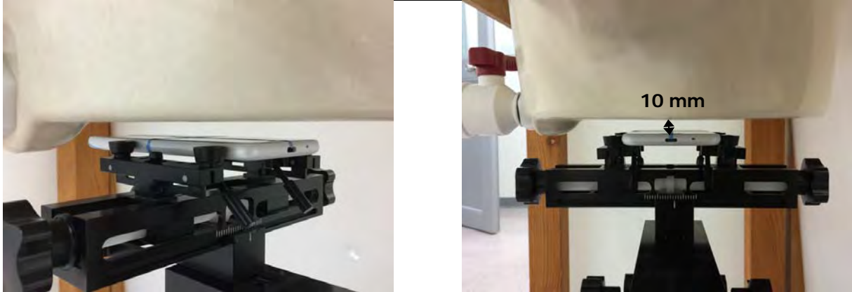
Fig.7 EUT Front side to flat phantom
