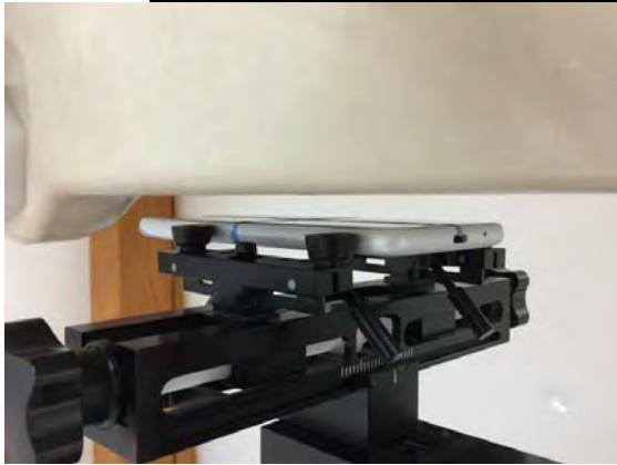
Fig.9 EUT Front side to flat phantom
