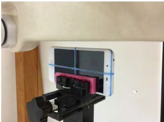
Fig.14 EUT Left side to flat phantom
