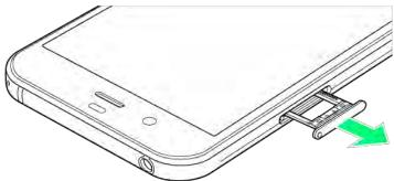
■ Do not pull SIM Tray forcefully or at an angle; damage may result. Gently pull it out horizontally by hooking a finger on it.
