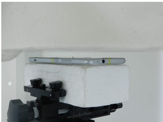
Front, Test Separation 10 mm
