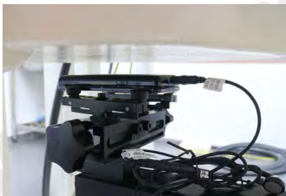
Fig.9 EUT back side with headset to flat phantom
