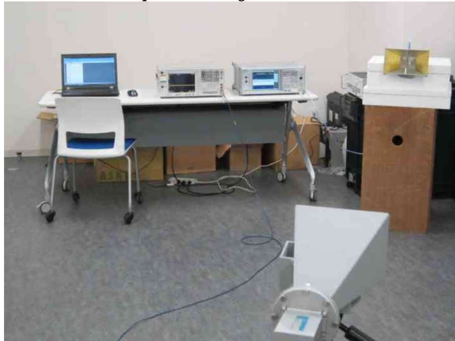
Test Setup for Generating the Radar Waveform
