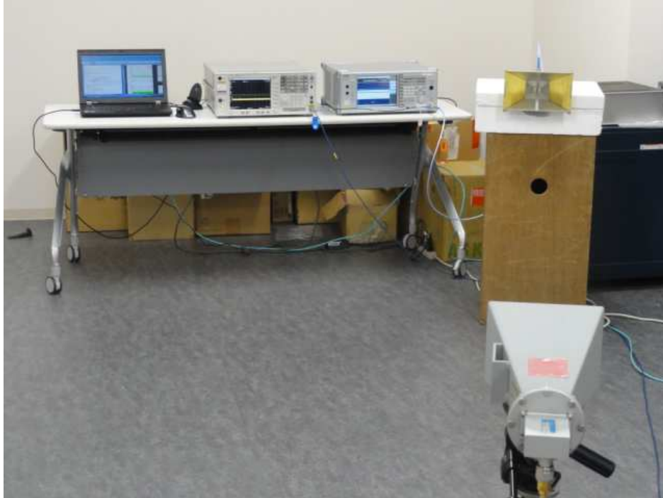
Test Setup for Generating the Radar Waveform
