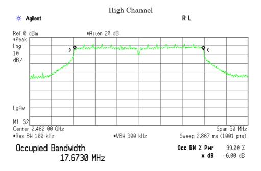
**Transmit Freq Error** 6.394 kHz **Occupied Bandwidth** 17.677 MHz
