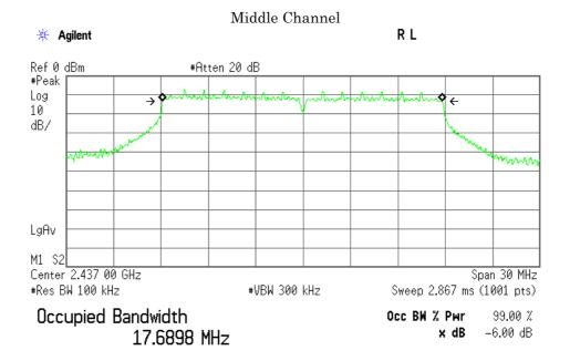
Transmit Freq Error -36.767 kHz Occupied Bandwidth 17.683 MHz
