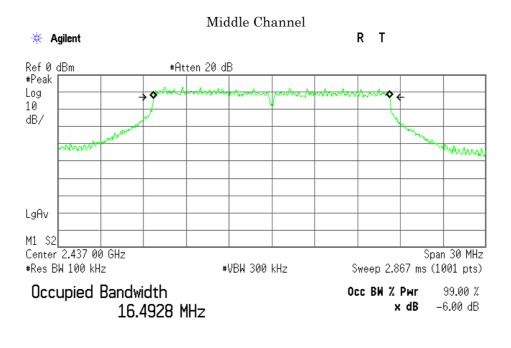
Transmit Freq Error -27.033 kHz Occupied Bandwidth 16.520 MHz
