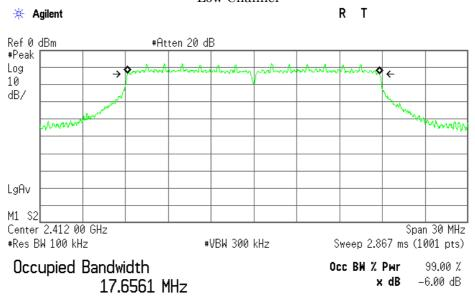
Transmit Freq Error -16.969 kHz Occupied Bandwidth 17.666 MHz
