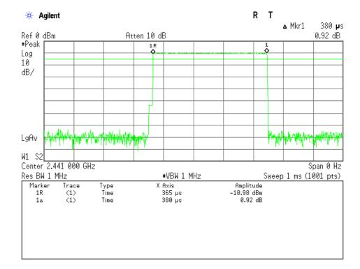
Note: The system makes worst case 1600 hops per second or 1 time slot has a length of 625  $\mu s$  with 79 channels. A DH1 Packet need 1 time slot for transmitting and 1 time slot for receiving. Then the system makes worst case 800 hops per second with 20 channels. So the system has each channel 40 times per second and so for 8 seconds the system have 320.0 times of appearance.
