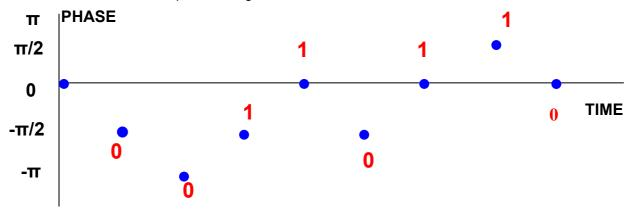
It would be preferable to have "gradual" changes in place between each pair of bits (Continuous-phase modulation). Replacing each "rectangular" shaped pulse (for 1 or 0) with a sinusoidal pulse can do this:
