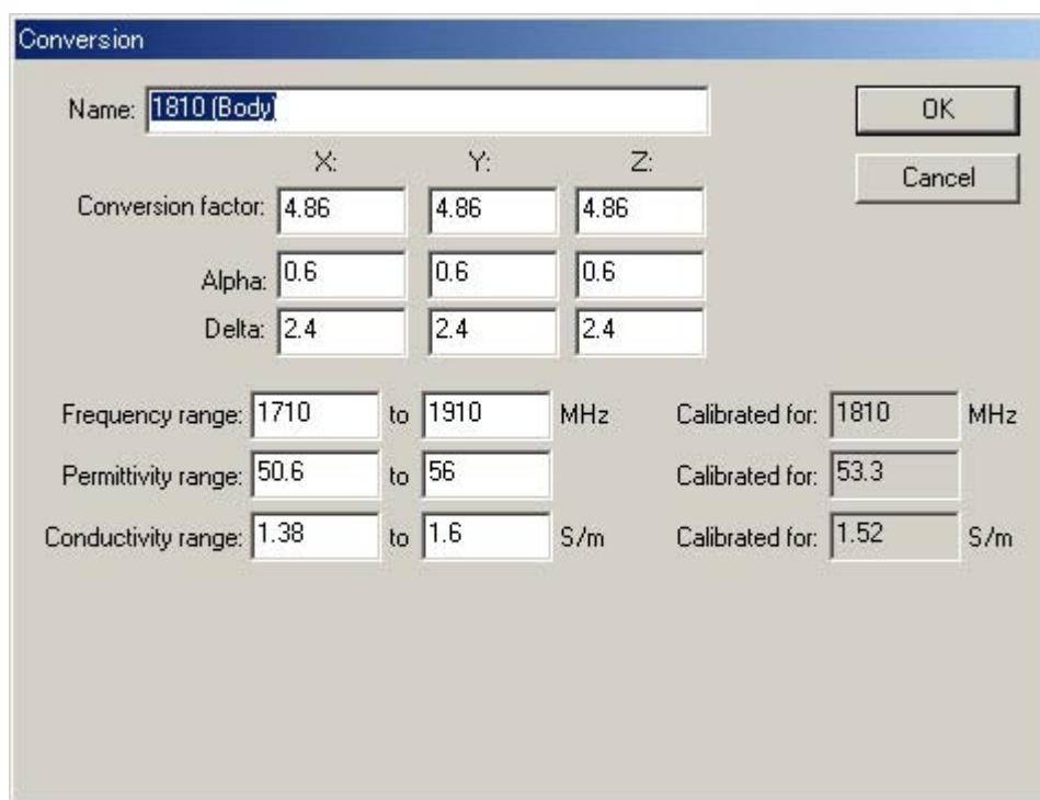
The target permittivity and conductivity at 835 MHz is 41.5 and 0.90 and 1900 MHz is 40.0 and 1.40 respectively which is within the calibrated range of the probe parameter. The following parameters are declared in the probe calibration certificate.
