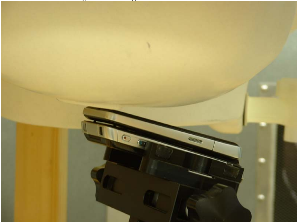
Configuration 4 (Right Head – Ear/Tilt Position)
