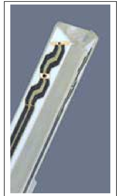
Inside view of ET3DV6 E-field Probe
