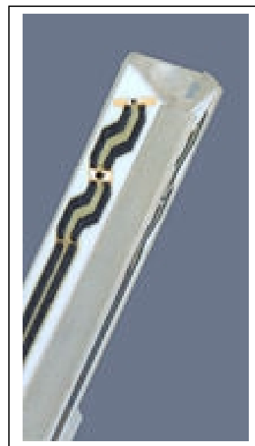
Inside view of ET3DV6 E-field Probe
