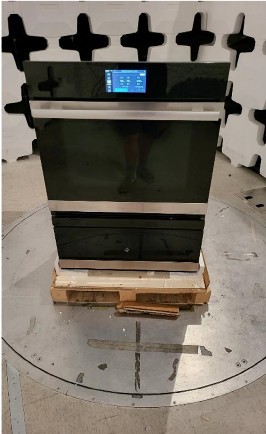
Figure 9. Photograph of Radiated Emissions Test Configuration, Close-Up
