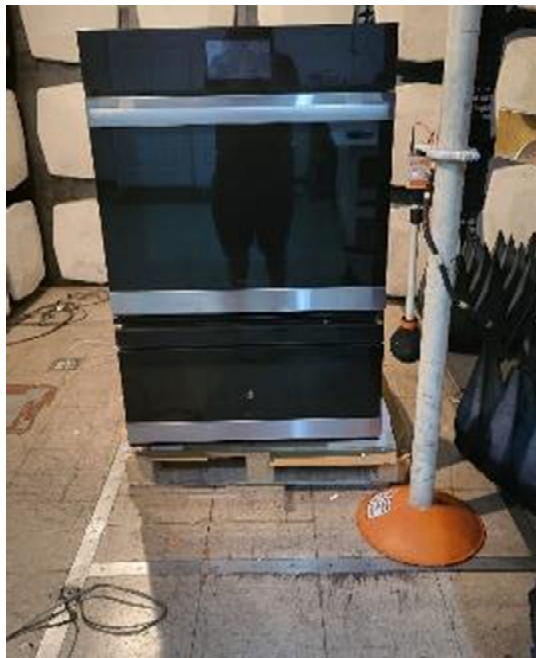
Figure 16. Radiation Leakage Setup
