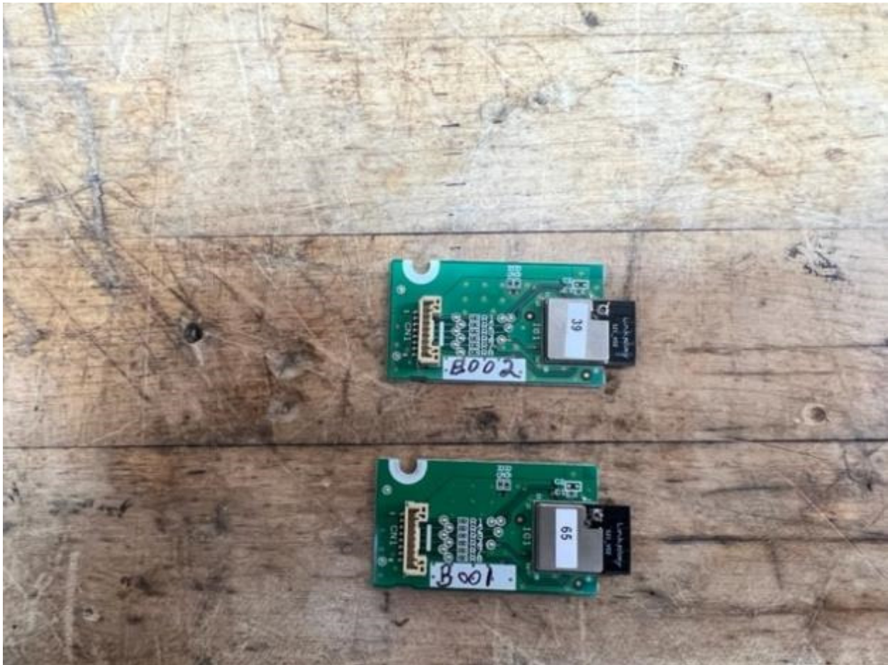
Figure 13. Wi-Fi modules on host interface boards, Top View
