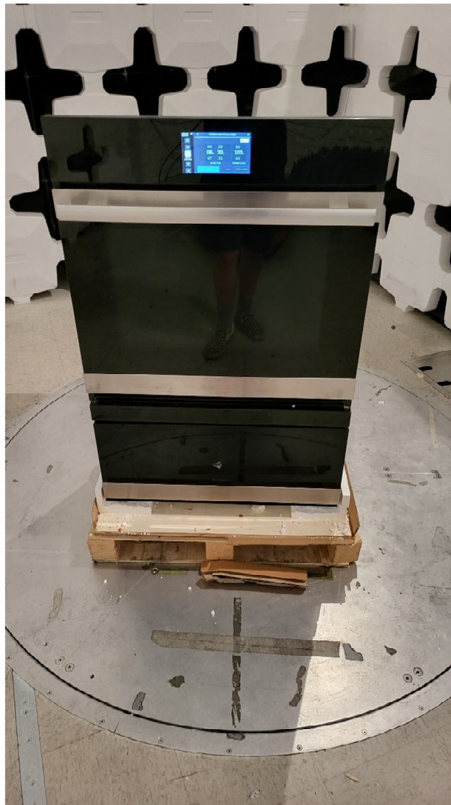
Figure 1. Radiated Emissions Measurement Photo (Front View)
