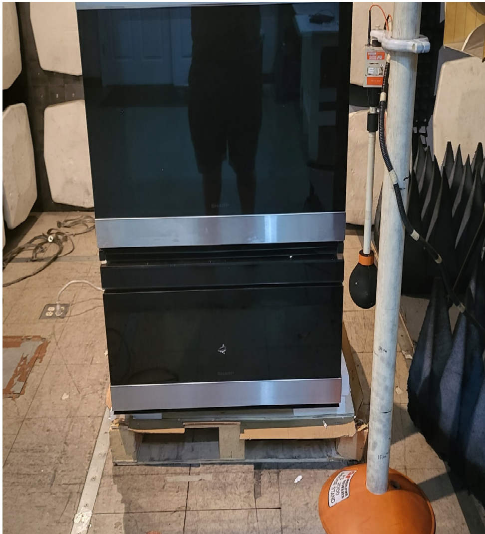
Figure 6. Radiation Leakage w/ RF Probe
