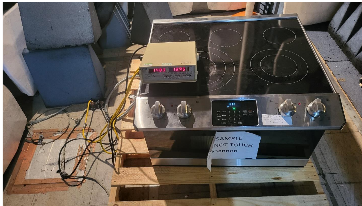
Figure 13. Input Power Test Setup
