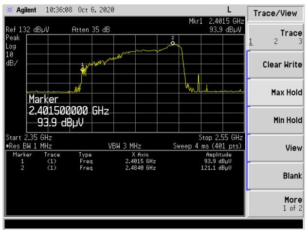
Figure 21. Frequency Variation at High Voltage -Tamura Switching Power Supply
