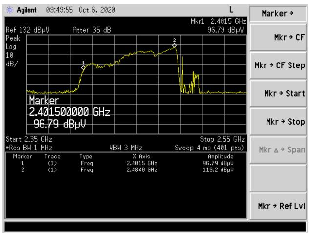
Figure 20. Frequency Variation at Low Voltage -Tamura Switching Power Supply
