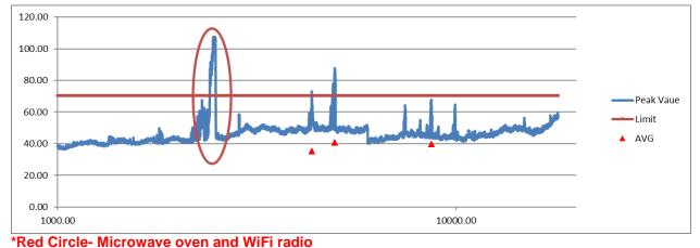
Figure 13. Vertical Antenna Position, 1 – 18 Ghz -Tamura Switching Power Supply
