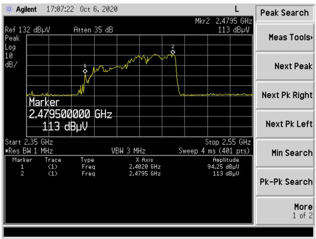
Figure 17. Frequency Variation at Low Voltage - Mitsuoka Switching Power Supply
