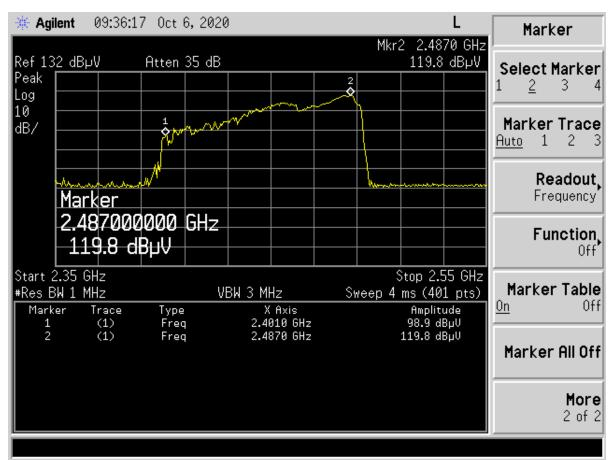
Figure 19. Frequency Variation at Nominal Voltage - Tamura Switching Power Supply
