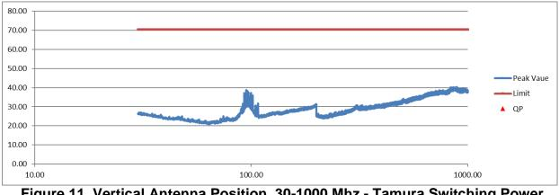
Figure 11. Vertical Antenna Position, 30-1000 Mhz - Tamura Switching Power Supply
