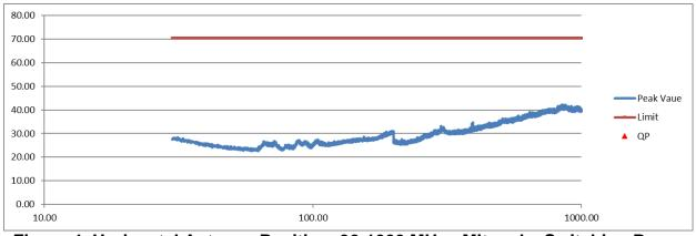
Figure 4. Horizontal Antenna Position, 30-1000 MHz - Mitsuoka Switching Power Supply
