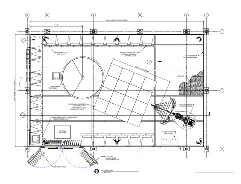
Figure 3. Radiated Emissions Disturbance Measurement Facility Diagram
