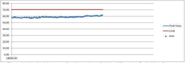
Figure 9. Vertical Antenna Position, 18 – 25 GHz - Mitsuoka Switching Power Supply
