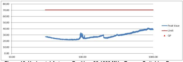
Figure 10. Horizontal Antenna Position, 30-1000 MHz -Tamura Switching Power Supply
