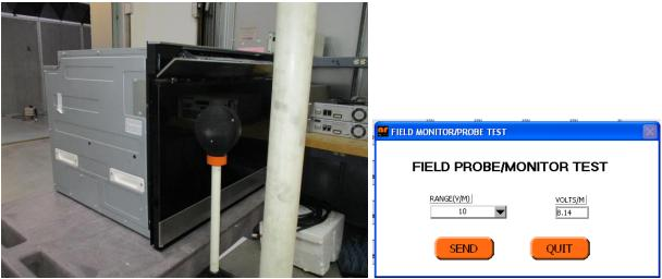
Figure 22. Leakage from Mitsuoka Switching Power Supply
