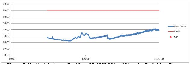
Figure 5. Vertical Antenna Position, 30-1000 MHz - Mitsuoka Switching Power Supply
