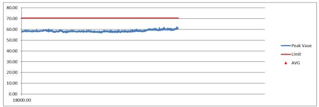
Figure 14. Horizontal Antenna Position, 18 – 25 Ghz - Tamura Switching Power Supply
