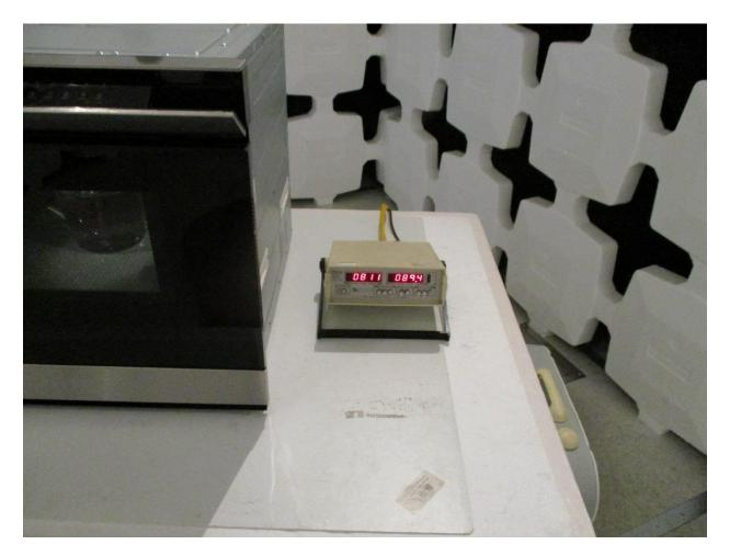
**Figure 6. Input Power Test Configuration (both Power Supplies)**
