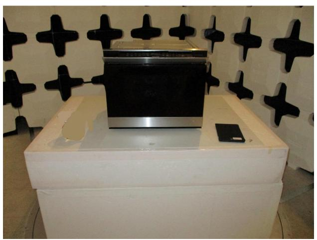
Figure 1. Radiated Emissions Measurement Photo Close-up (both Power Supplies)
