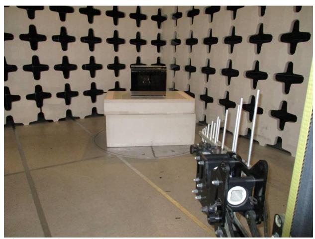
Figure 3. Radiated Emissions Measurement Photo, 200 to 1000 MHz (both Power Supplies)
