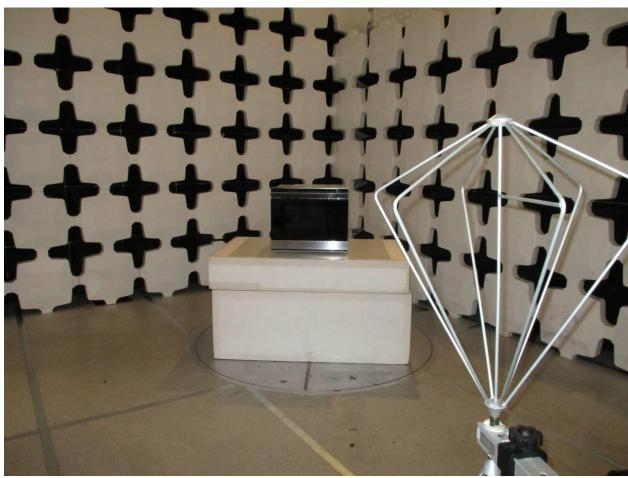
Figure 2. Radiated Emissions Measurement Photo, 30 to 200 MHz (both Power Supplies)
