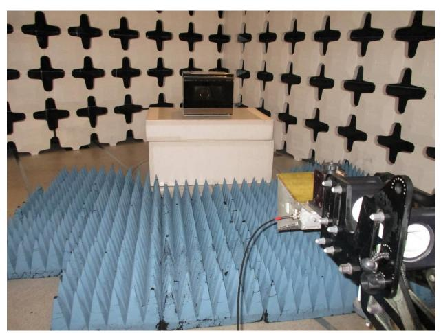
Figure 4. Radiated Emissions Measurement Photo, above 1000 MHz (both Power Supplies)
