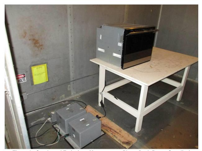
Figure 8. Conducted Emissions Measurement Photo (both Power Supplies)
