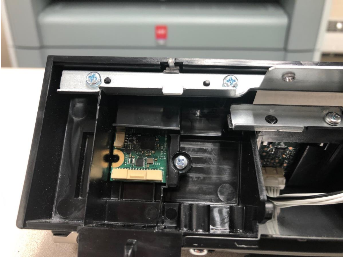
Figure 12. Wi-Fi Module Location in Microwave
