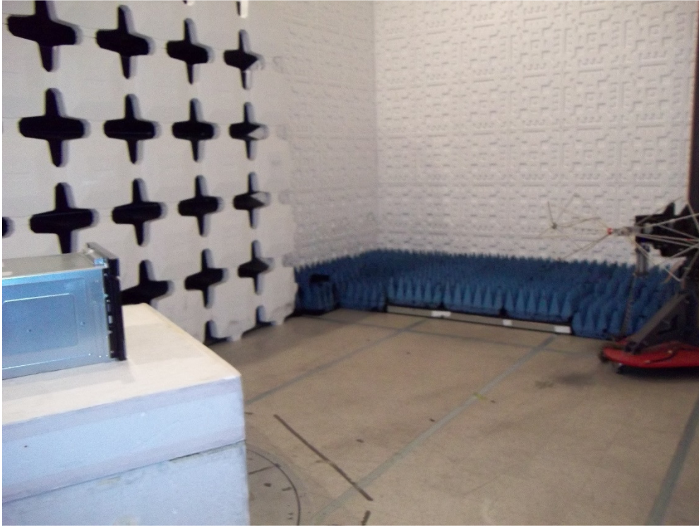
Figure 10. Photograph of Radiated Emissions Test Configuration, 30 - 200 MHz
