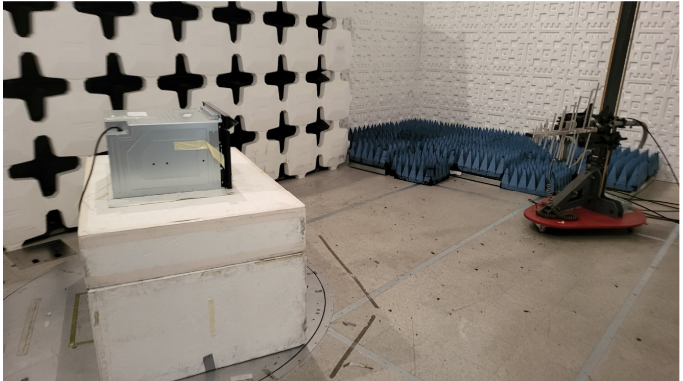
Figure 11. Photograph of Radiated Emissions Test Configuration, 200 - 1000 MHz
