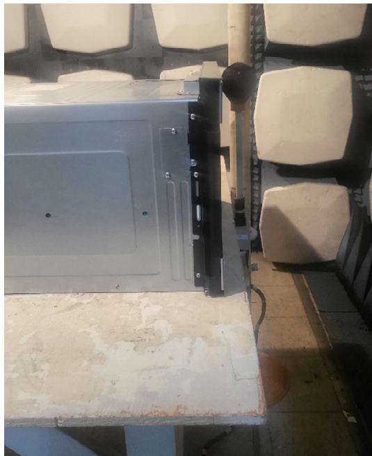
Figure 16. Radiation Leakage Setup
