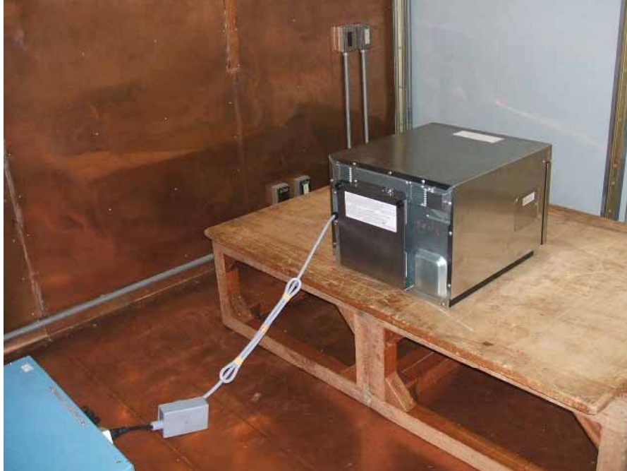
Photograph present configuration with maximum emission
