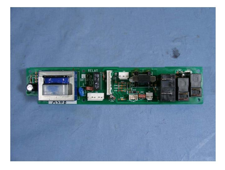
Photographs of appliance Fig. 9 Shows back-side of relay unit PWB assembly.
