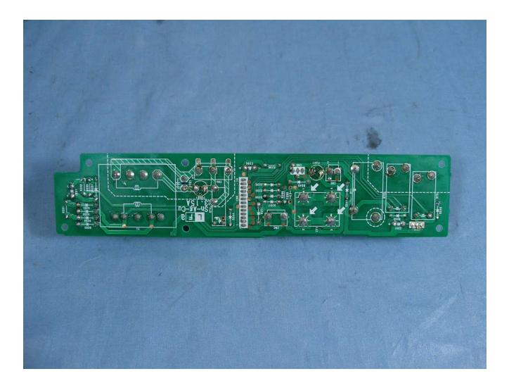
Photographs of appliance Fig. 10 Shows control unit PWB assembly.
