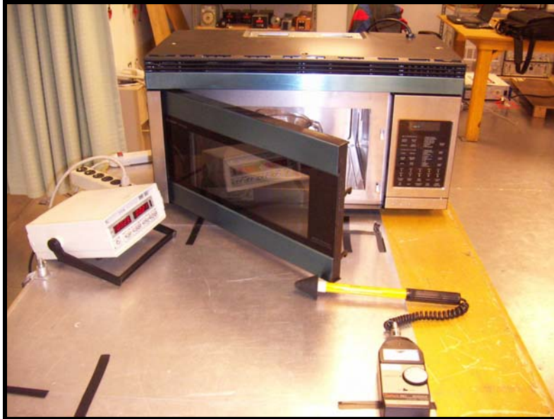
Radiation Hazard Measurement
