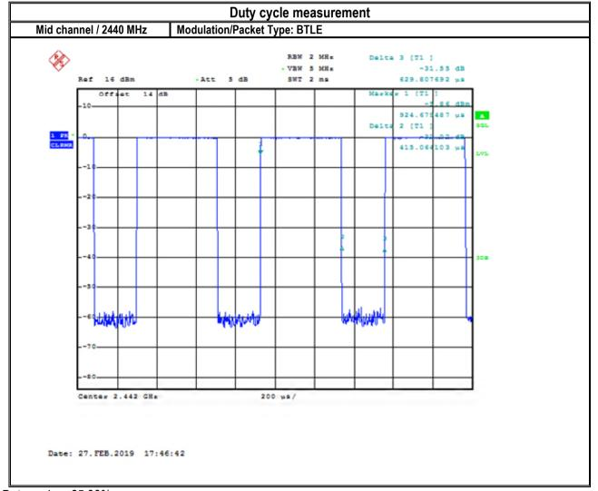
Duty cycle = 65.90% Duty cycle correction factor =10\*log (1/0.6590) = 1.81 dB
