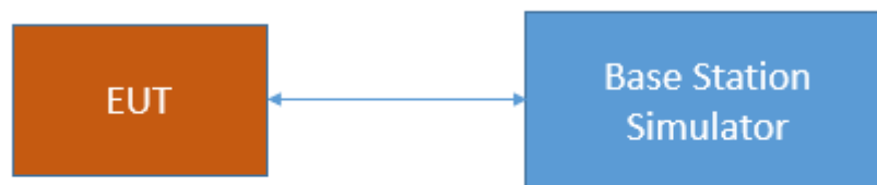
Test Setup FCC Part 22/24/27/90 Cellular; Frequency stability
