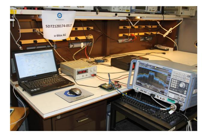
Antenna Conducted Port Test Setup
