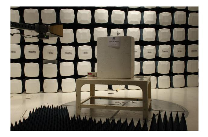
Radiated Emissions Test Setup (above 1GHz)
