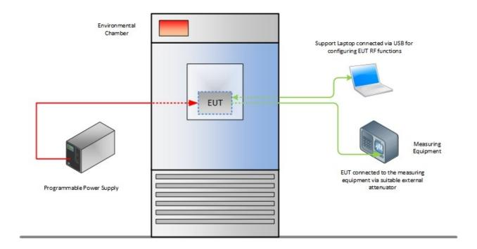
**Frequency Stability Test Configuration**
