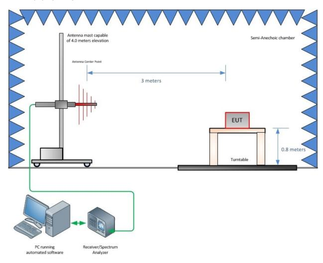
Radiated Emission Test Setup (Below 1GHz)
