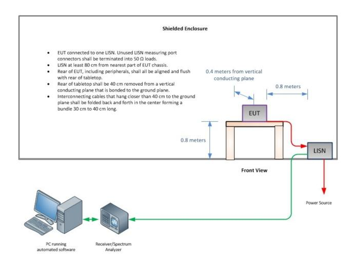
**Conducted Emissions Test Configuration (if applicable)**
