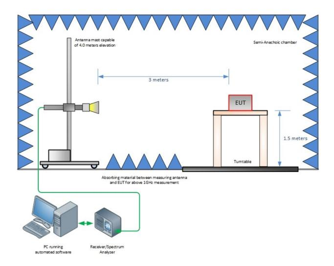
Radiated Emission Test Setup (Above 1GHz)
