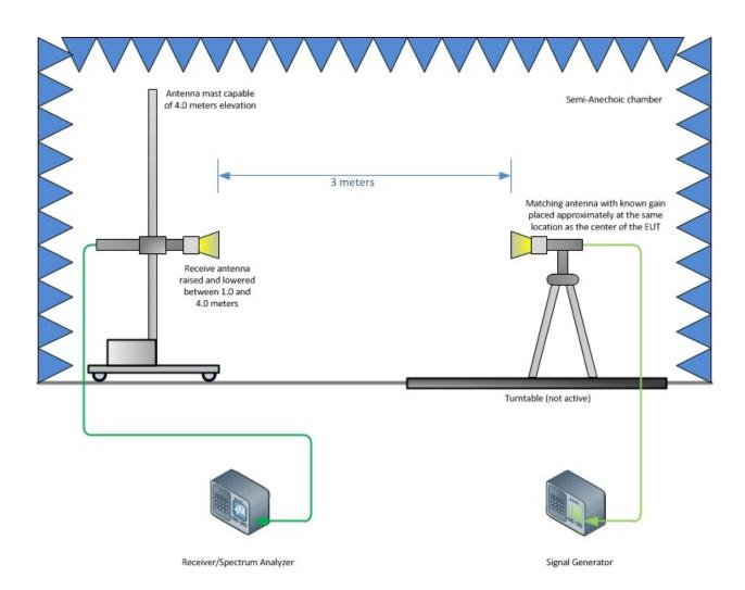
Substitution Test Method (Above 1GHz, if applicable)
