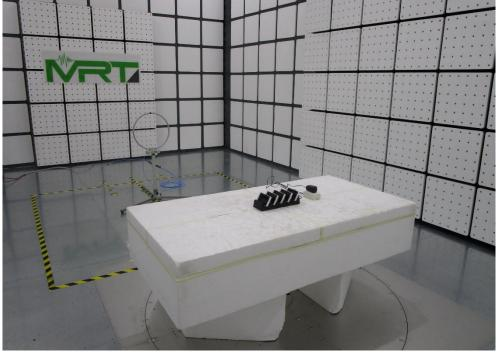
Test Mode: Mode 1 Description: Radiated Emission Test Setup for 30MHz ~ 1GHz
