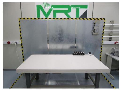
Test Mode 1 Description: Back View of Conducted Emission Test Setup
