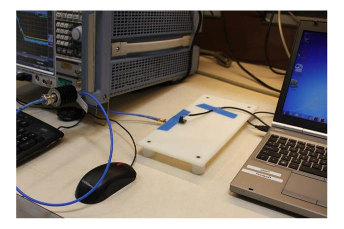
Antenna Conducted Port Test Configuration
