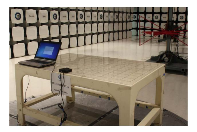
Radiated Emissions Test Setup (below 1GHz)
