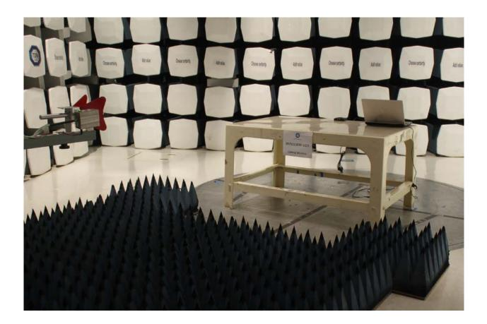
Radiated Emissions Test Setup (above 1GHz)
