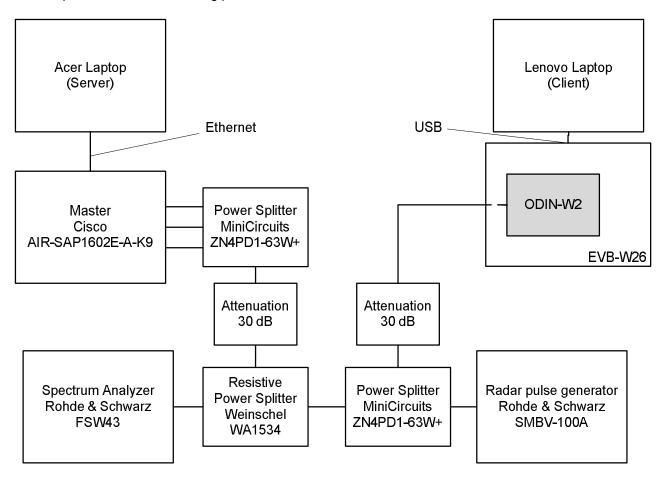
The second rf-port is for MIMO operation in WLAN 2.4 GHz only and disabled at 5 GHz. Therefore only the main rf-connector was used for these tests.
