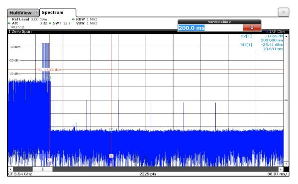
The beacons after the channel closing transmission time of 200 ms are additional intermittent control signals caused by the master (See Note 2 in 4.5).
